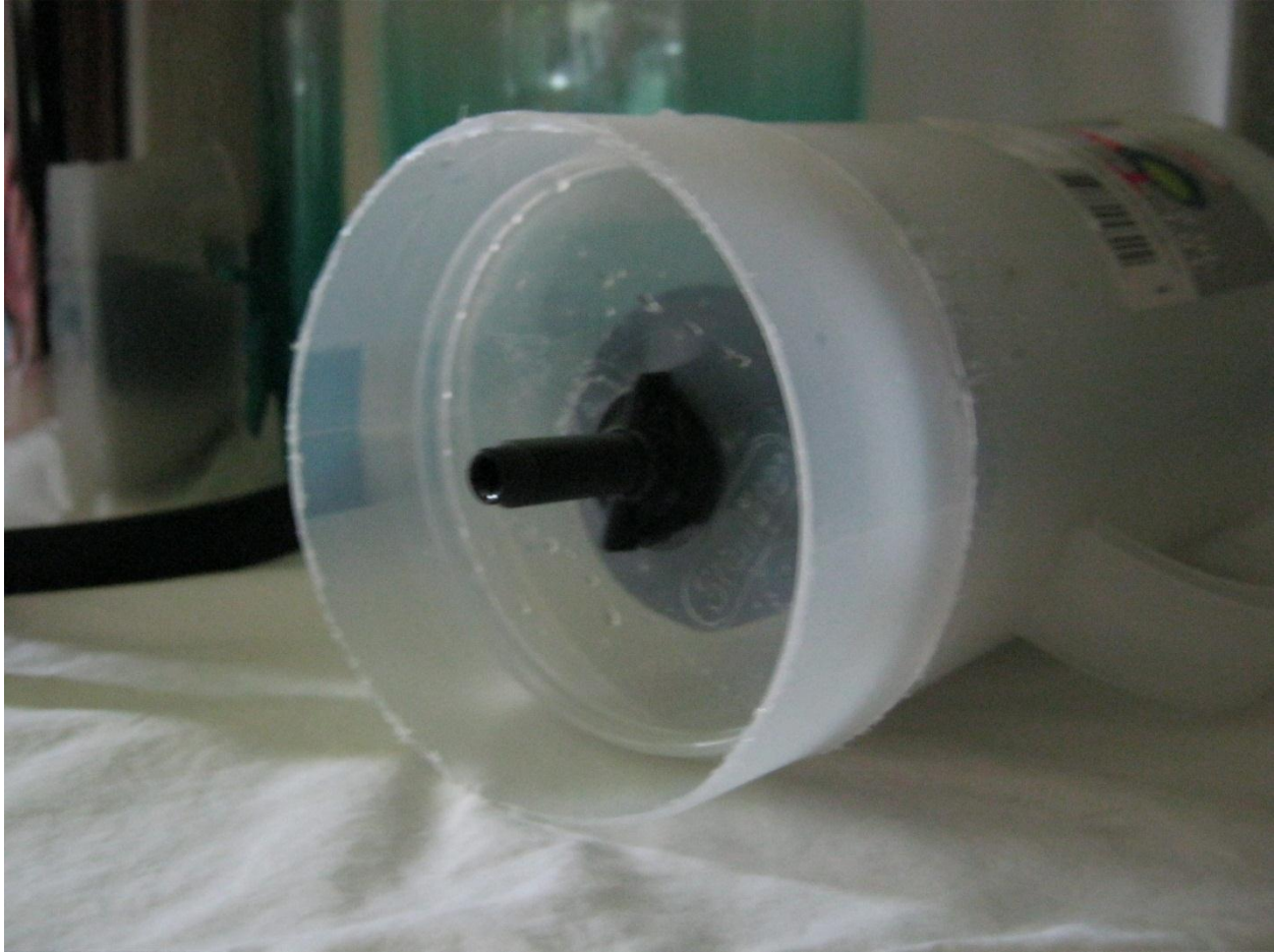
Bottom of top chamber with filter in place and improvised adapter
