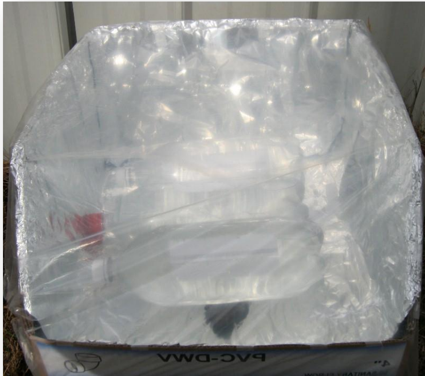
The finished product - note front of box cut at an angle and bottles inside
